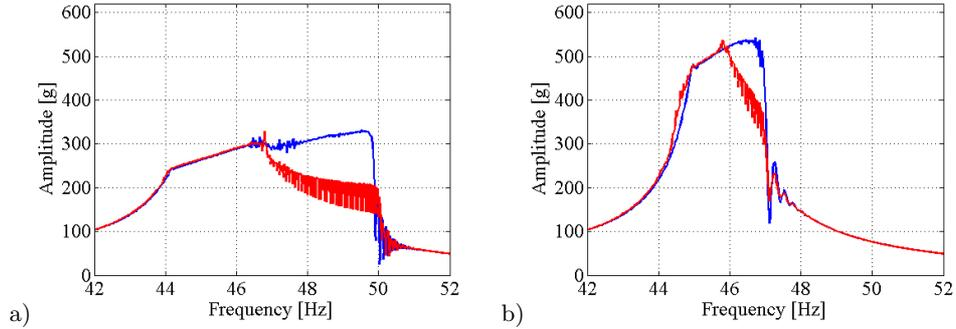
**Figure 3.** Amplitude of inertial acceleration output versus frequency at different gap sizes between beam and stopper: 6.5mm (a) and 11mm (b). The blue and red lines correspond to up and down frequency sweep, respectively. Note that we limited the discussion to the first mode shape of beam vibration.
