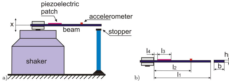
**Figure 1.** Experimental stand (a), Note the location of the piezoelectric patch, and accelerometer (sensor). Characteristic dimensions of the excited aluminum beam (b). To minimize the risk of fracture of the piezoceramic element we placed the thin layer of rubber on the stopper.
