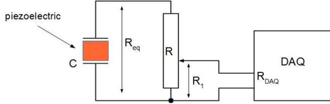
**Figure 2.** Electrical circuit set with the electro-motive force on the piezoceramic element; the circuit of the voltage divider was used in order to adjust the measured voltage to the range available for the DAQ card.
