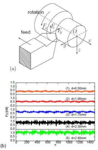
**Fig. 1.** (a) The schema of a turning process. The three orthogonal measured force components: feed  $F_x$ , thrust  $F_y$ , and cutting  $F_{z'}$  (b)  $F_y$  time series of the stainless steel turning process versus sampling number n for five different cutting depths d (referred in the text as the cases (1)–(5)). The sampling frequency was chosen at 2 kHz.
