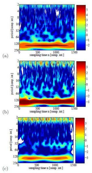
**Fig. 3.** Wavelet power spectra  $P_W$  for different cutting depths d = 1.00, 1.75, 2.30 for a, b, and c; respectively (cases (2)-(4) in Figs. 1b and 2b). The colours are related to the magnitudes of  $P_W(s, n)$  according to the logarithmic scale  $\log_2$  (see right panels marked with the corresponding scale exponents). The total measurement time of N = 1500 samplings is related to 0.75 sec.
