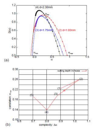
**Fig. 2.** (a) Multifractal bands of the three chosen cases (2)–(4) from the Fig. 1b. (b) The complexity diagram  $\alpha_{top}$  versus  $\Delta \alpha$  with all examined process denoted by numbers (1)–(5) (as in Fig. 1b).
